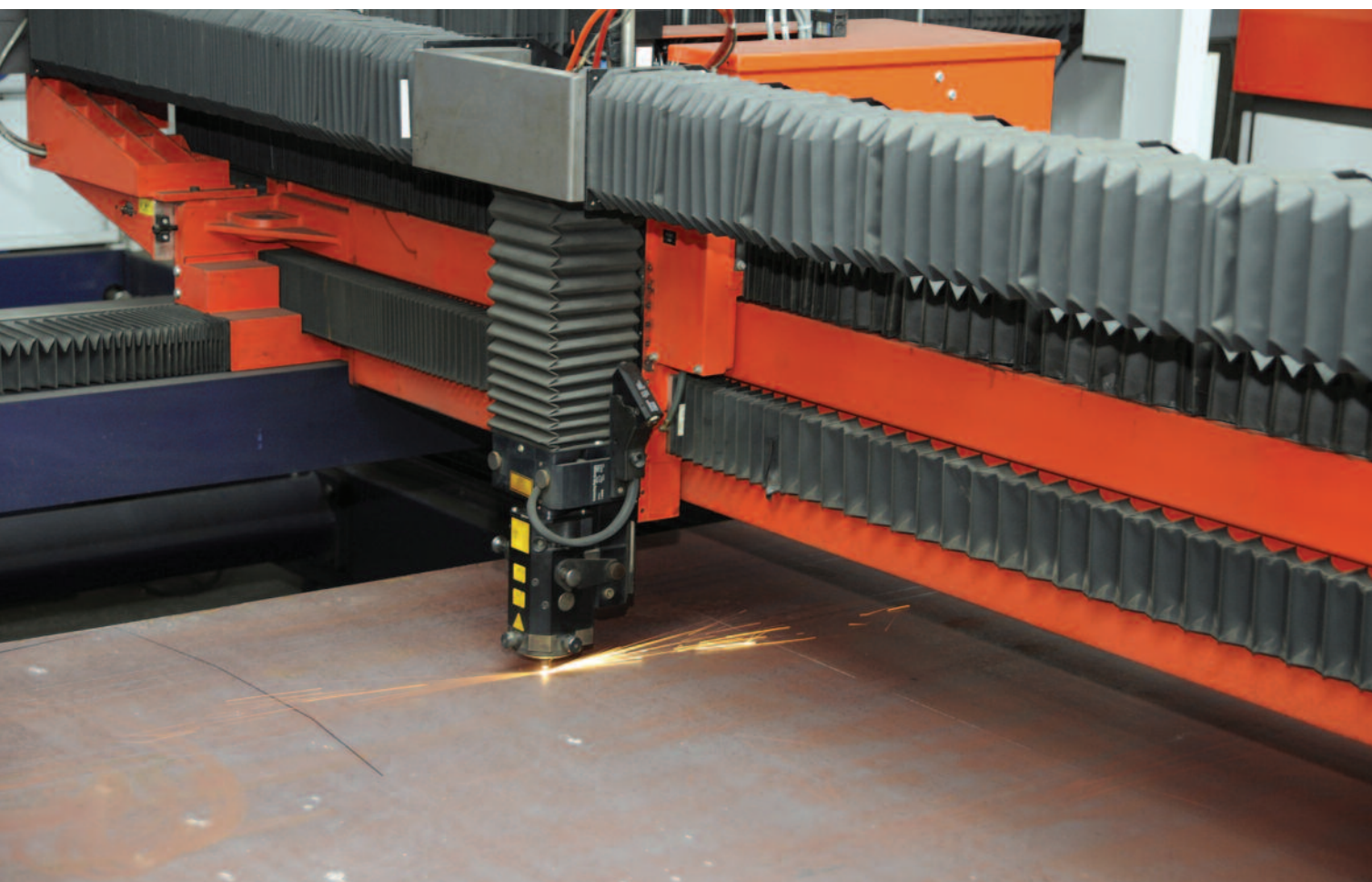
Components of high-tech laser cutting machines are protected by bellows fabricated from materials made by Dickson PTL.
