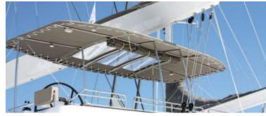
he practical application of photovoltaic fabrics has taken an important step forward with the introduction of a bimini top that not only blocks the sun, but also generates enough power to recharge on-board batteries or power small electronics. Catamaran builder Lagoon, Dickson-Constant and Nv Equipment debuted the application during the Cannes International Boat and Yacht Show this past fall aboard the 62-foot Lagoon 620.
